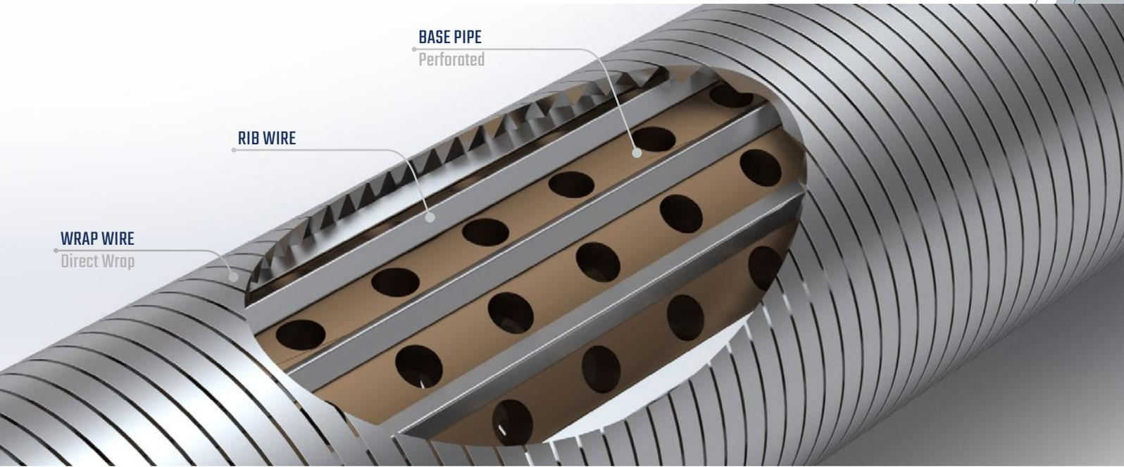
Capture is a robust Direct Wrap on pipe screen designed for stand alone and gravel pack sand control applications. The profile/shaped wire is wrapped directly on the *base pipe* providing conformance and eliminating the gap between screen and *base pipe*. This process creates a unified structure producing enhanced mechanical properties such as collapse, burst, bend, tensile, compression and torque superior to conventional slip-on WWS.
