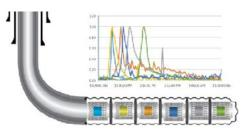
Tracers are placed in the string, with a unique signature for each Zone. Two types of Tracer are available, one which is water activated, and thus can be used with the unique signature to identify and quantify the water producing zone, and the other is an Oil Contact Tracer which is used to quantify the rate of Oil Production.
